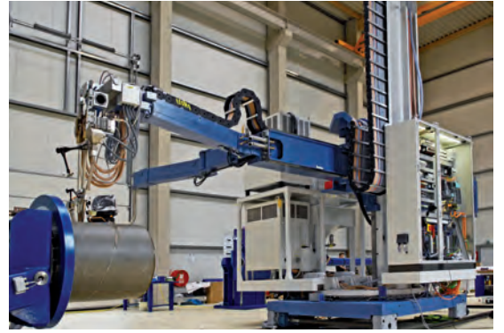
Outside Welding Column
