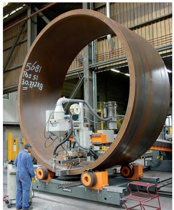
Inside welding column – Flux handling system Wind tower production (Offshore)
