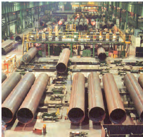
Large diameter pipes, welded with high-performance welding equipment
